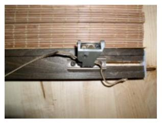
Insert a screwdriver into the cord lock to keep the gears open and then pull the wire and the cord up between the gears. The cord lock has three compartments separated by wire. Make sure the cords go in the outer compartments - one in each.
