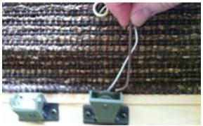
It is easiest to cord through the cord lock if you attach a thin piece of wire to the end of the cord.
