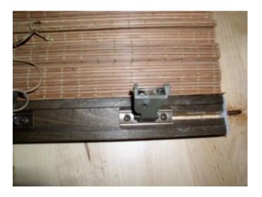
Step 6: Re-thread the new cord lock. Pull the cord through the front of the cord lock and straight out the back. Do not push up through the gears yet.
