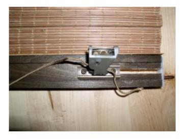
Step 7: Attach wire to cord to help you thread the cord through the gears.
