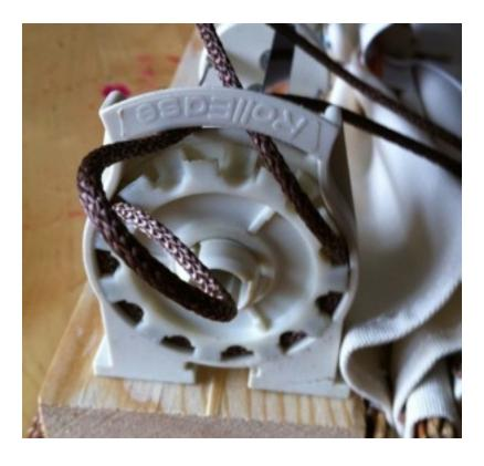
Once the cord is all the way out, simply remove by pulling it under the Roll Ease tab and away from the clutch. To install the new cord, simply perform the operation in reverse. First pass the cord under the Roll Ease tab:
