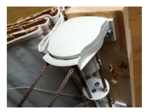
To remove the cover, insert a screw driver under the inside end of the clutch and release the tab which is holding the cover on. Do not try to remove the cover by releasing the tab at the other end of the cover (underneath the Roll Ease sign). Only release the cover as shown in the photo and it should pop off easily.
