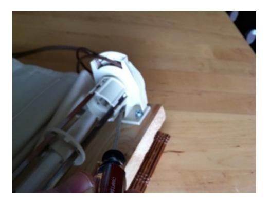
Now the gear wheel and the cord are exposed at the end of the clutch.
