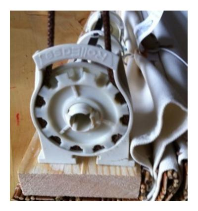
To remove the cord, simply pull the cord through between the gear wheel and the Roll Ease tab and then turn the gear wheel gently and pull the cord out.
