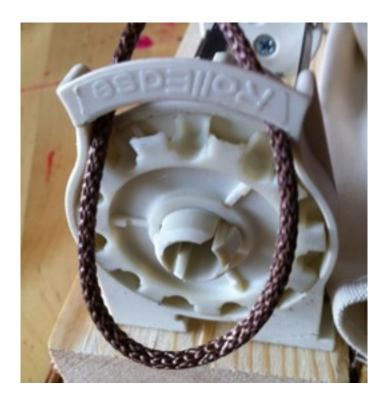
and then engage it with the gear wheel and keep turning until the cord runs all the way around the gear wheel:
