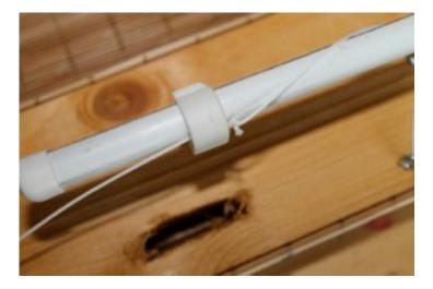
Once the knot reaches the clip, remove the clip and then reattach it with the knot on the other side of the clip. Make sure the cord runs through the slit in the clip. Make sure the clip is aligned with the others and the same distance as the others from the bracket.
